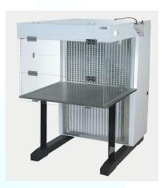
germicidal UV tube. Side panels are of safety flexi glass 6 mm in thickness mounted with anodized aluminum angles. Front door of perplex sheet with anodized aluminum frames and locks having arrangement to work with half open door. Hepa Filter facing to working table is being well protected with a grill pf perforated aluminum material.
